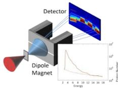
**Particle detector development** The ultra-short and high fluence particle bunches from the source have to be detected and evaluated. Key parameters are particle yield per energy slice and peak energy. The expected reduction of bunch length requires additional developments for ultra-fast high-resolution detectors with repetition rate capability in the Hz range.
